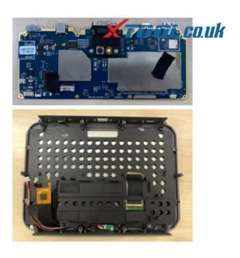
Step 6: Tighten the screws to fix mainboard and battery
