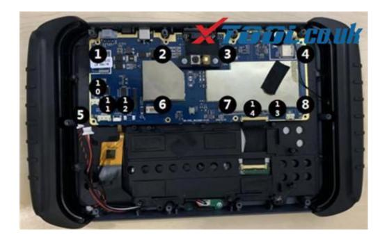
Step 5: Loosen the screws (No.1~No.8)
