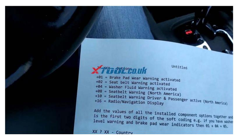
The number in the third position here is what region your car is in and this determines what units your car uses whether it's kilometers or miles Celsius or Fahrenheit and whether it uses a 12 or 24 hour clock system.
