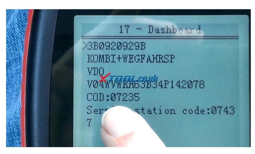
So a quick word about what these numbers mean: the numbers in the first two position indicate what warnings you want on and it works by adding these numbers up and what I mean by that is like if you wanted brake Pad wear warning and seatbelt warning, only you would do 1\*2 equals 3 and so the number right here would be 03.
